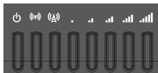
Figure 2 - NTC-140W-02 router LED Indicators
